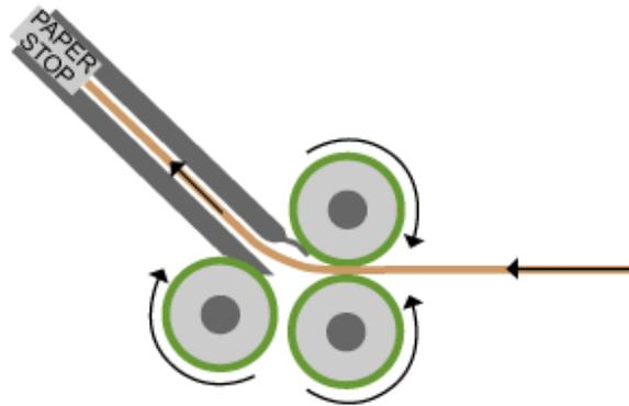
When the paper strikes the backstop, it buckles and is forced downward and into a set of nip rollers.
