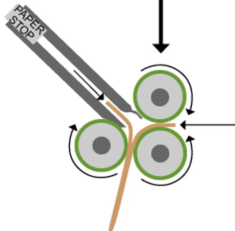
A combination folder, as the name implies, provides both close registration and a higher speed for folding. The combination folder is used most often for large quantities and more complex folding jobs.
