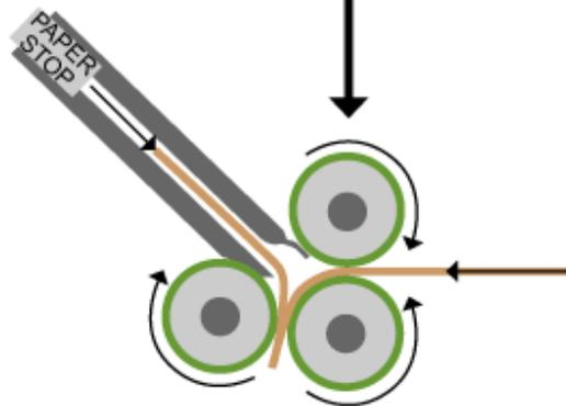
The nip rollers grab the sheet at the buckle and pull it through, compressing a fold into the sheet as it passes through the rollers. If several folds are desired, then the material is sent into another plate to repeat the process. The fold or buckle location is adjustable by altering the stop mechanism. This allows for different folds to be created depending upon the type of fold required.
