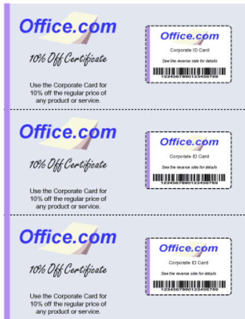
A 3-up direct mailer with a horizontal perforation for bursting, following the laser personalization of the copy.
