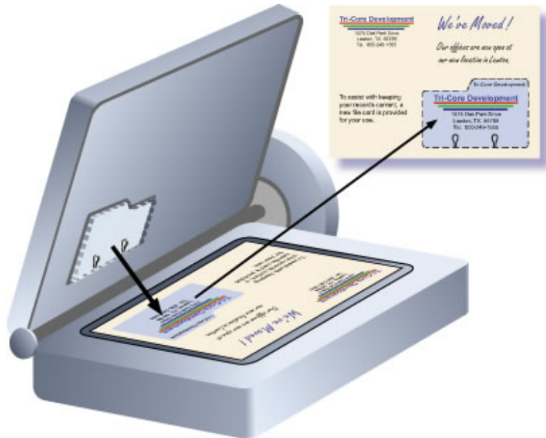
A platen press can be used to apply a complicated perforation to an application. As shown in the example above, this method is often used for applying the perforation that surrounds a removable card.
